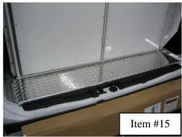
Place trim panels as shown above Pre-drill through trim panel (only) with 3/16". Pre-drill the vehicle w/ 1/8" hole and attach panels using #10 x 1" sheet metal screws
